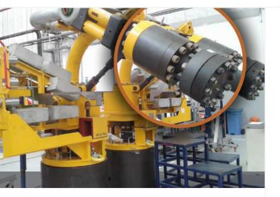
DSTI subsea swivels reduce installation time and equipment stress by allowing flexible flowlines to rotate up to 360 degrees.
