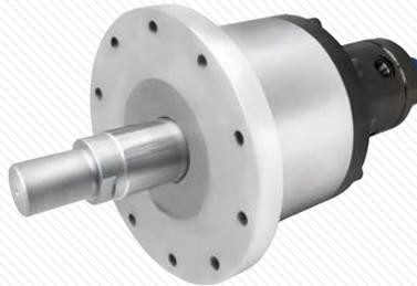
**Specialized Example 2** - designed for an uncoiler / recoiler expanding mandrel application. Design features a complete assembly solution integrating a rotary union, rotating cylinder (for actuating the expanding mandrel), and position sensor.
